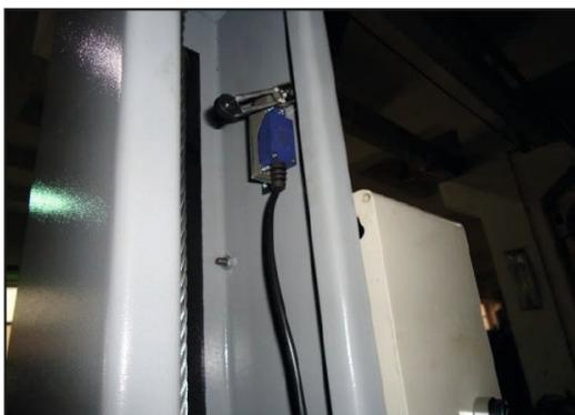
Figure 19 (upper end limit switch)
